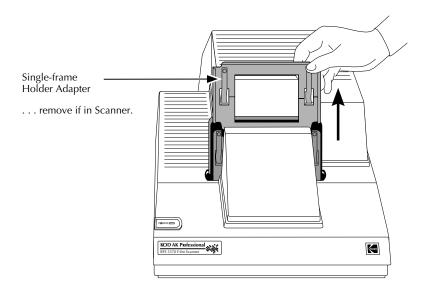
2. If the 35 mm multi-frame holder adapter is not in the Scanner, put it in place in the Scanner in the orientation shown.
